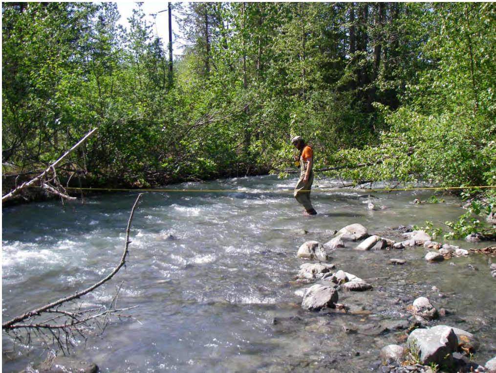
Photo 12. Discharge measurement taken on Falls Creek during June, 2009.
